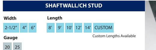
Used in shafts containing elevators, ducts, piping, air shafts and similar construction applications.
